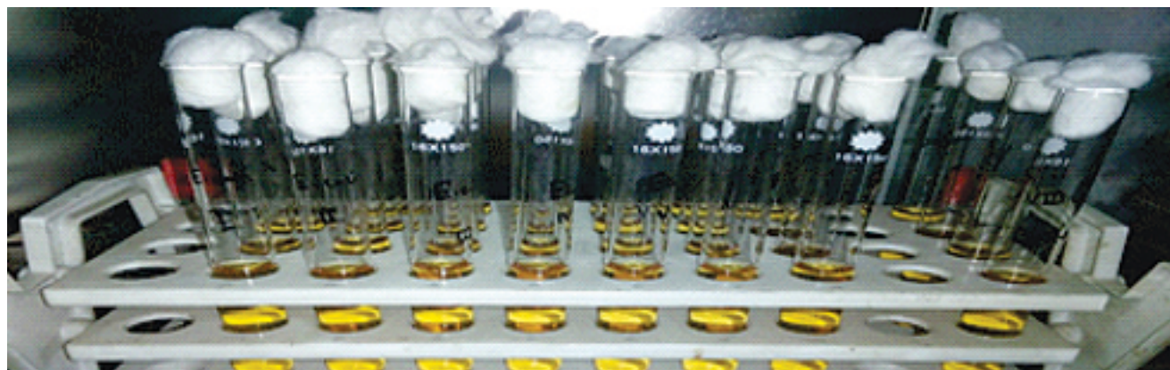
Figure 4: Determination of Minimum Inhibitory Concentration (MIC) of amikacin by broth dilution technique.
